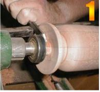
Dish Out the top flange with a parting tool to create a cradle for the candle.
