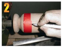
Determine the circumference of the spindle by wrapping masking tape around it and drawing a line across the overlapping pieces.
