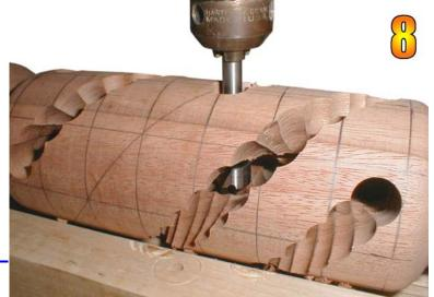
These candle holders also have a couple of big brothers. To make these 4" by 4' spirals, I mounted the drillpress on a carriage that rolls across the lathe bed.
