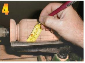
Use a flexible straightedge to draw the spiral layout lines.
